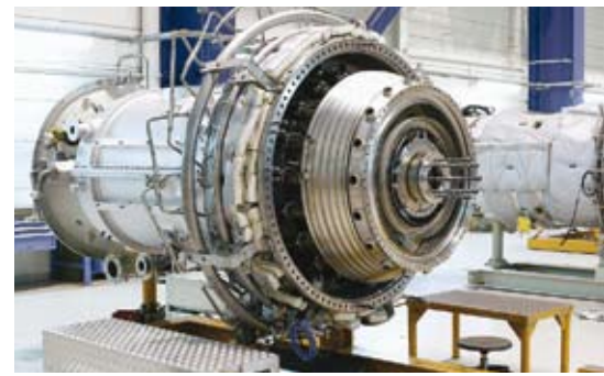
SGT-700 gas generator.
